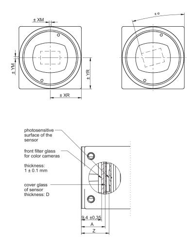
Figure 10 Sensor accuracy of the Baumer VEX series
