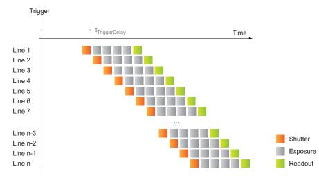
For cameras with rolling shutter sensor and set shutter mode Rolling, for each frame each line begins exposure at an offset equal to each line's readout time. The exposure time for each line is the same, but the start and end times are staggered. Data readout for each line begins immediately following the line's exposure. The readout time for each line is the same, but the start and end times are staggered.
