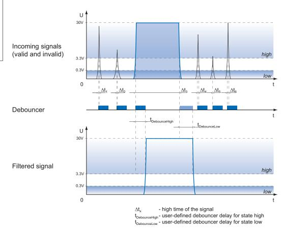
Please note that the edges of valid trigger signals are shifted by  $t_{DebounceHigh}$  and  $t_{DebounceLow}!$
