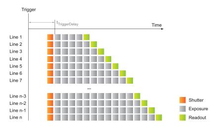
For cameras with rolling shutter sensor and set shutter mode Global Reset, for each frame all of the lines start exposure at the same time but the end of exposure is delayed by the offset of the previous line's readout. The exposure time for each line gradually lengthens. Data readout for each line begins immediately following the line's exposure. The readout time for each line is the same, but the start and end times are staggered.
