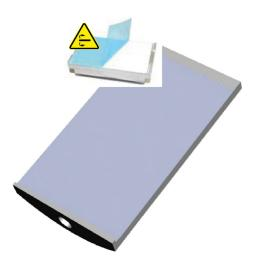
2. Place the clamp element with the adhesive tape on the top side of the camera.
