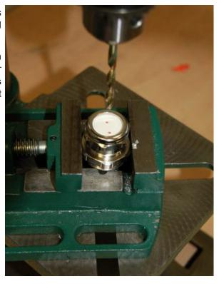
**3.** After drilling, slit the seal insert radial from the holes to the outside, using a sharp cutting knife.
