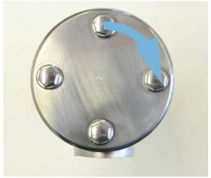
**4.** Tighten the screws crosswise only so far that the light blue cover seal is flush with the surface of the housing.
