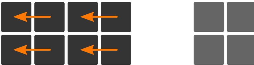
**Figure 8.3:** Monochrome Sum-type horizontal binning
