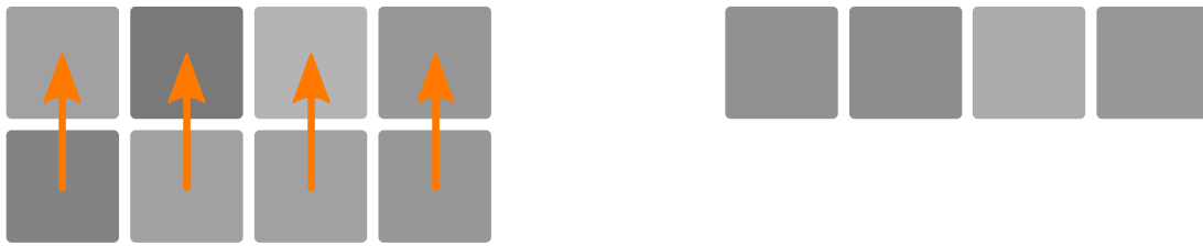
Figure 8.7: Monochrome Average-type vertical binning
