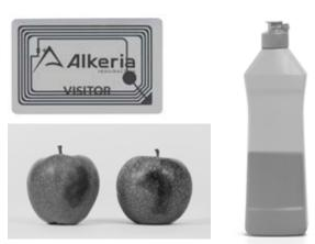
Examples of what a SWIR camera can capture: e. silicon, bruising inspection, fluids level inside opaque bottles.
