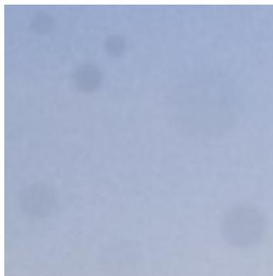
**Figure 3.12:** Example of lens or filter impurities
