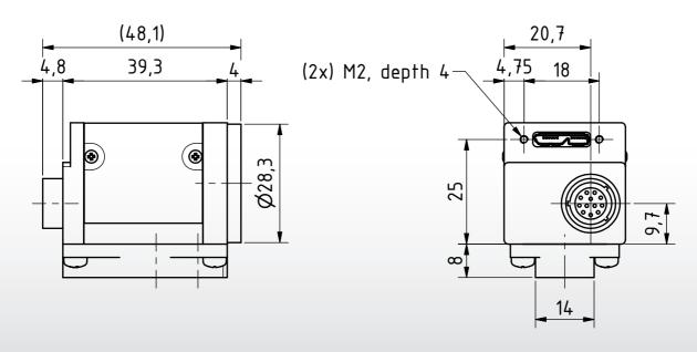
Dimensions: mm Tolerances: DIN ISO 2768m
