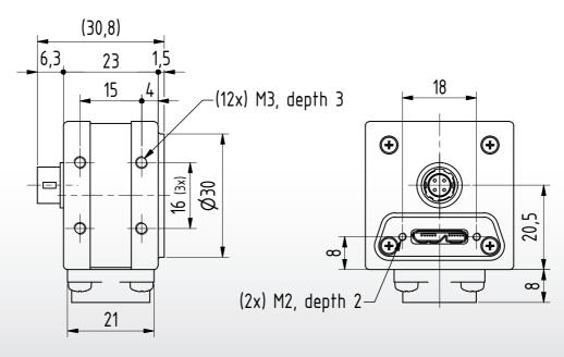
Dimensions: mm Tolerances: DIN ISO 2768m
