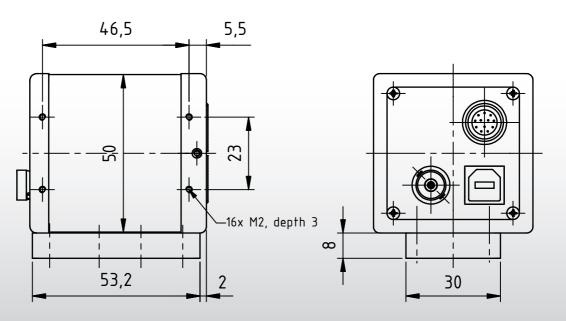
Dimensions: mm Tolerances: DIN ISO 2768m
