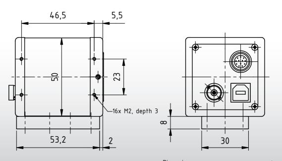
Dimensions: mm Tolerances: DIN ISO 2768m
