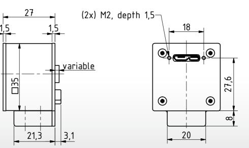
Dimensions: mm Tolerances: DIN ISO 2768m
