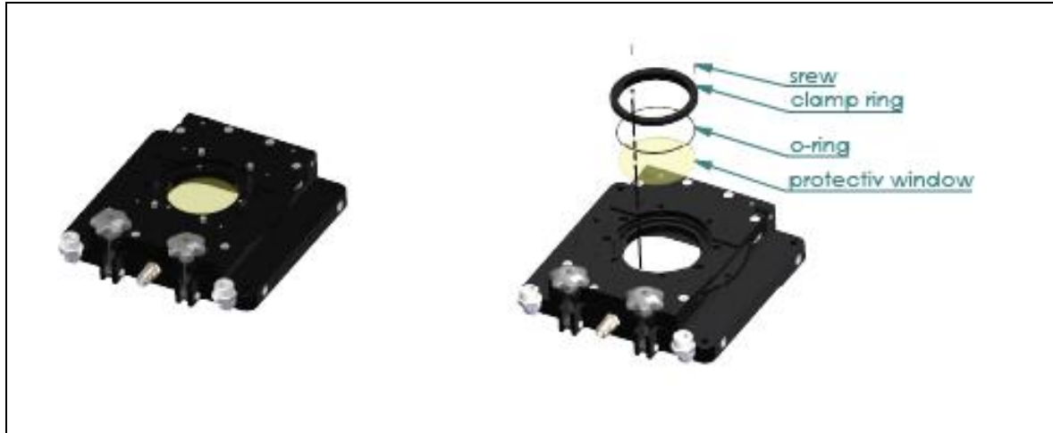
Figure 29: Change of the protective window
