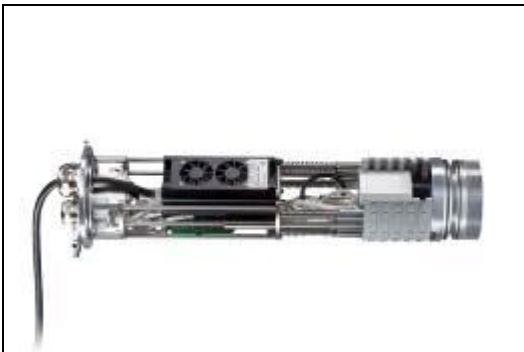
Figure 56: Cooling Jacket Advanced (Extended) with PI NetBox and industrial PIF
