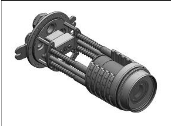
Figure 39: Front part with infrared thermometer
