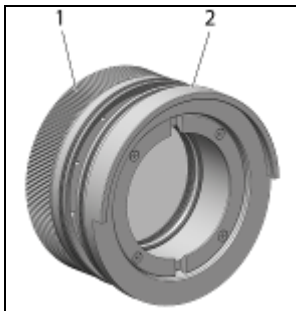
Figure 17: Focusing unit (external and internal part)
