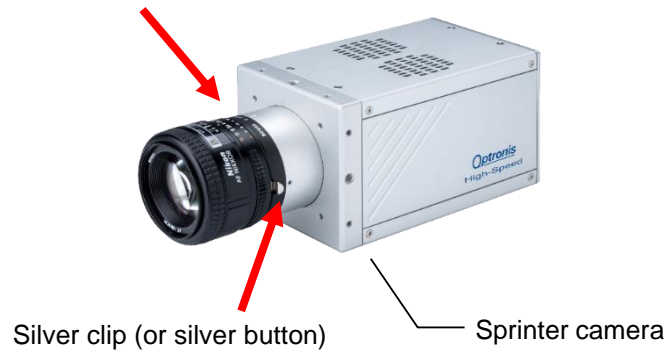
Figure 3: Overall Camera and lens view
