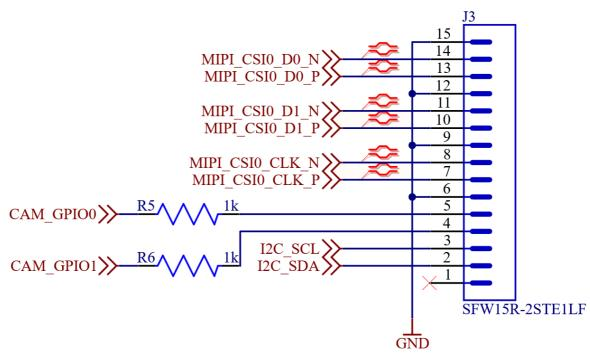
The CAM\_GPIOs and I2C-bus signals have the I/O voltage of 3.3V.
