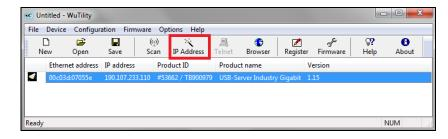
8. The standard setting of the USB server is DHCP. On a direct connection to a PC set a static IP address to the device. Take care that the network part of the address is identical to the network part of the IP address of the connected PC (therefore: **192.168.0**). The host part must have a different digit than the user-defined IP address of your PC (for example: 192.168.0.2):
