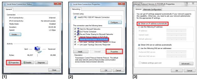
4. In the register card General enable the checkbox Obtain an IP address automatically [3]
