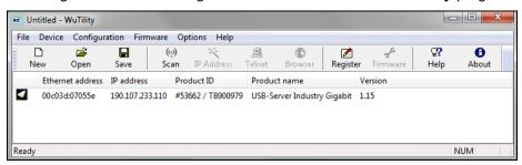
Independent on the current network settings of the USB server the device is displayed now (if not, refresh the current view with Scan).
