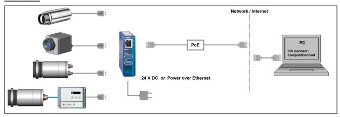
On a connection to a PC both over the network, the USB server as well as the PC must use an automatic IP address. Here the DHCP server is available. Review the following settings on your PC once (depending on the operating system the procedure can differ from the here shown – the following description refers to a Windows 7 system).
