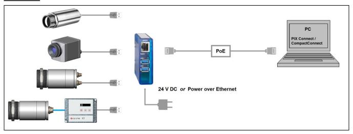
On a direct connection to a PC both, the USB server as well as the PC must use a fixed IP address. There is no DHCP server available. Accomplish the following settings on your PC once (depending on the operating system the procedure can differ from the here shown – the following description refers to a Windows 7 system).
