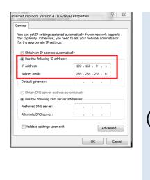
If you want to switch between a user-defined IP address and a DHCP server, the following alternative configuration is recommended: Under the General tab choose Obtain an IP address automatically, and on the Alternate Configuration tab, click User configured and enter a user defined IP address:
