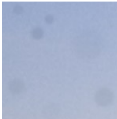
Figure 3.15: Example of lens or filter impurities
