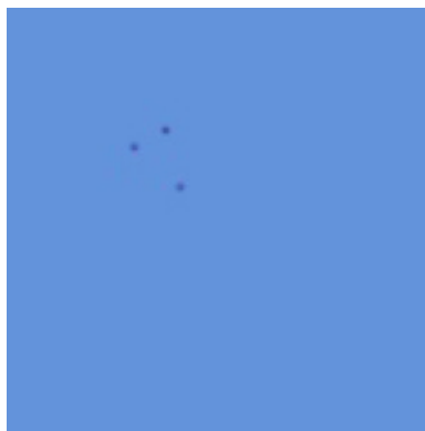
Figure 3.16: Example of sensor impurities
