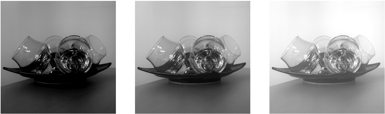
Figure 9.10: Black level calibration examples
