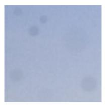
Figure 3.12: Example of lens or filter impurities
