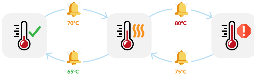
Figure 3.14: Temperature status transition
