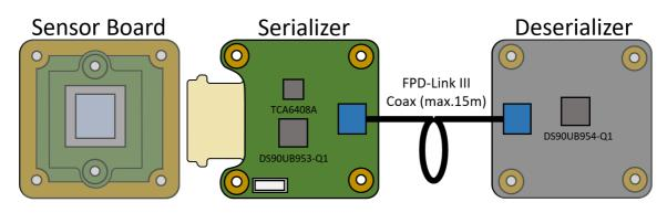
The document "Deserializer Design Recommendations" contains important information required to create a custom deserializer design using the TI DS90UB954-Q1 chip.
