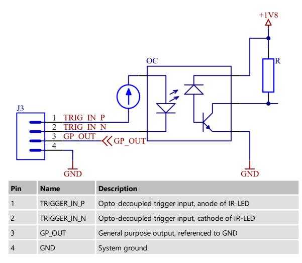
The trigger input is opto-decoupled. To drive the trigger input, voltage must be applied to pins 1 and 2. Note: pin 1 is the positive input; pin 2 is the negative input.
