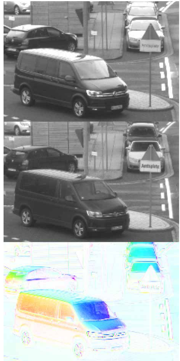
Fig. 12: Top image: Image from standard sensor showing heavy surface reflection. Center image: Image from four-directional polarizing sensor with reflections eliminated. Bottom: image with color mapping
