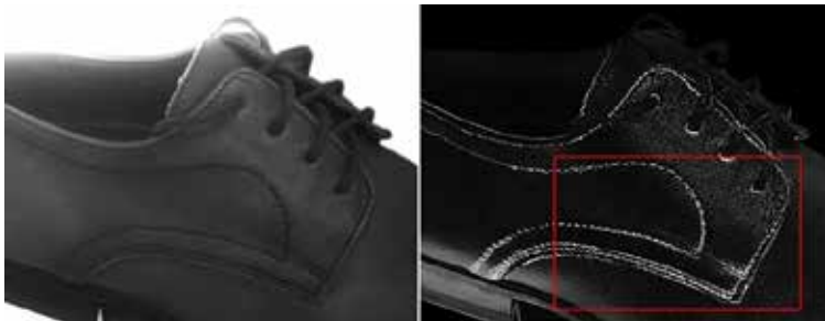
Fig. 5 (left): Left image made with standard imaging sensor. On the right, DoLP processing of the polarization data dramatically improves the contrast between the leather and stitching.
